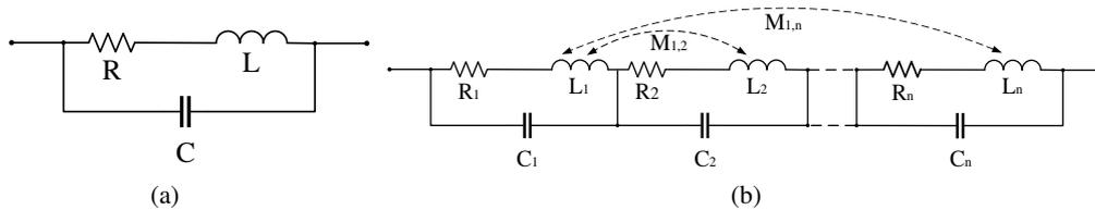
Fig. 1. The models of solenoid winding: simplified single unit RLC model (a); equivalent circuit of detailed model (b)
