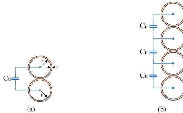
Fig. 3. The simulation geometry for calculating turn-to-turn capacitance (a), and the internal capacitances of one unit consisting of  $n_t = 4$  turns (b)
