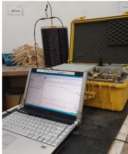
Fig. 9. FRA measurement setup
