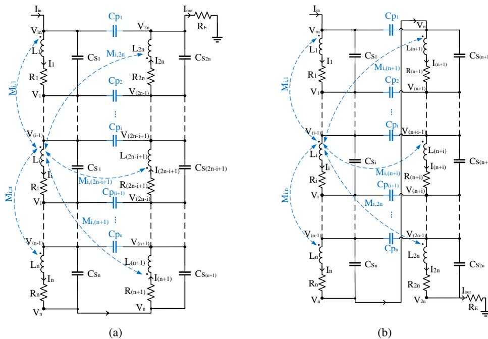
Fig. 2. The detailed model of the first (a) and second (b) test windings
