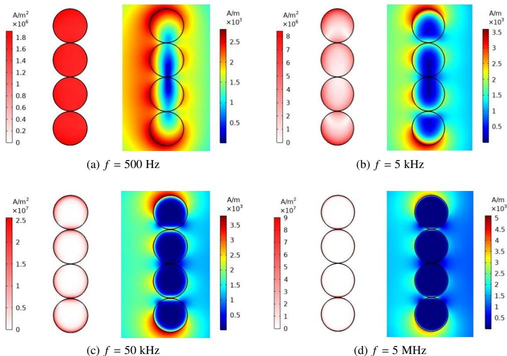
Fig. 6. The current density distribution across the conductors of a unit (left column), and the magnetic field at different frequencies (right column)
