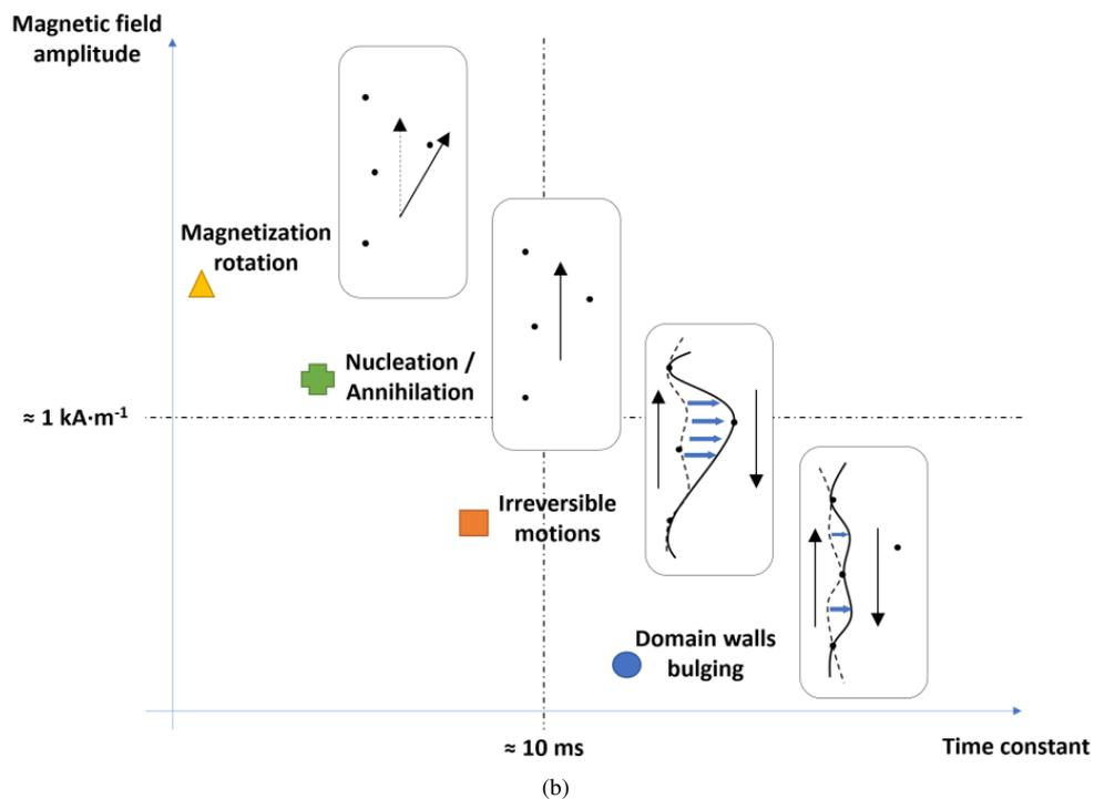
Fig. 1. Magnetization mechanisms, illustration graphic (a); magnetic field amplitude vs. time constant distribution of the magnetization mechanisms (b)
