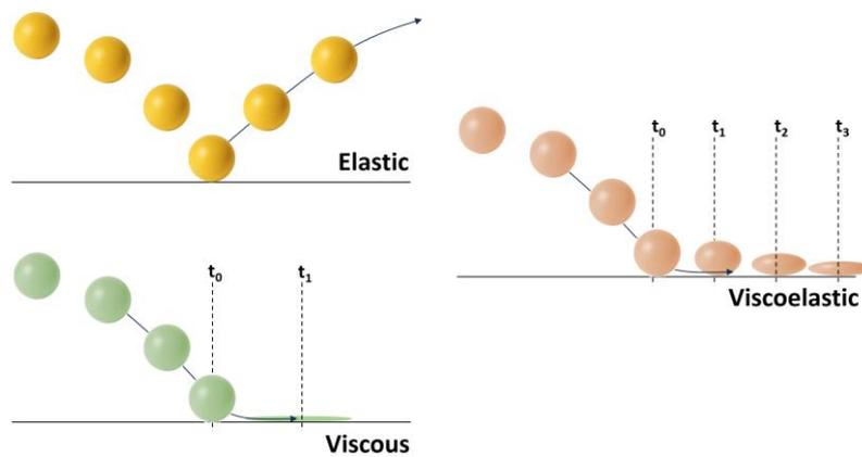
Fig. 2. Viscoelasticity: an illustration in a mechanical context
