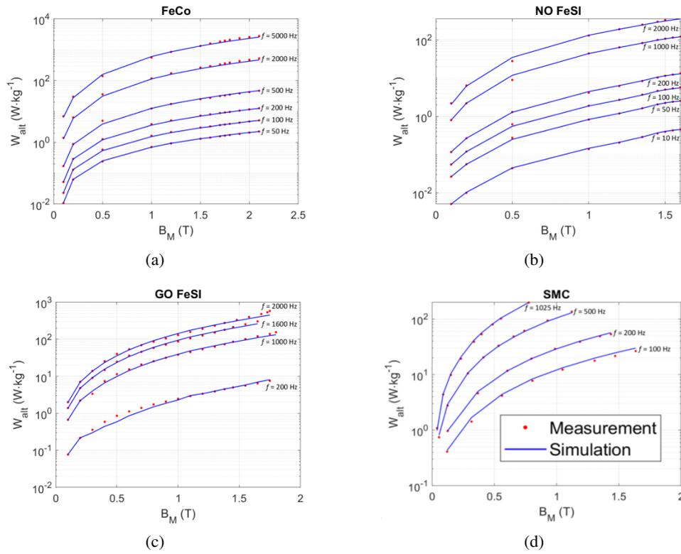
Fig. 3. Comparison between simulation and measurement under alternating unidirectional magnetization for four classical ferromagnetic materials: FeCo (a); NO FeSi (b); GO FeSi (c); SMC (d)
