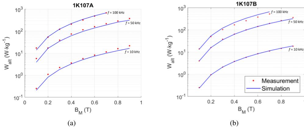
Fig. 4. Comparison of the magnetic power loss between simulation and measurement under alternating unidirectional magnetization for the 1K107A (a) and the 1K107B (b) nanocrystalline materials
