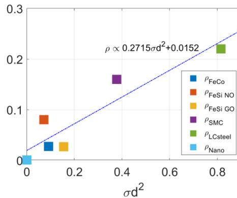
Fig. 5.  $\rho$  vs.  $\sigma d^2$  and linear fit for all tested materials
