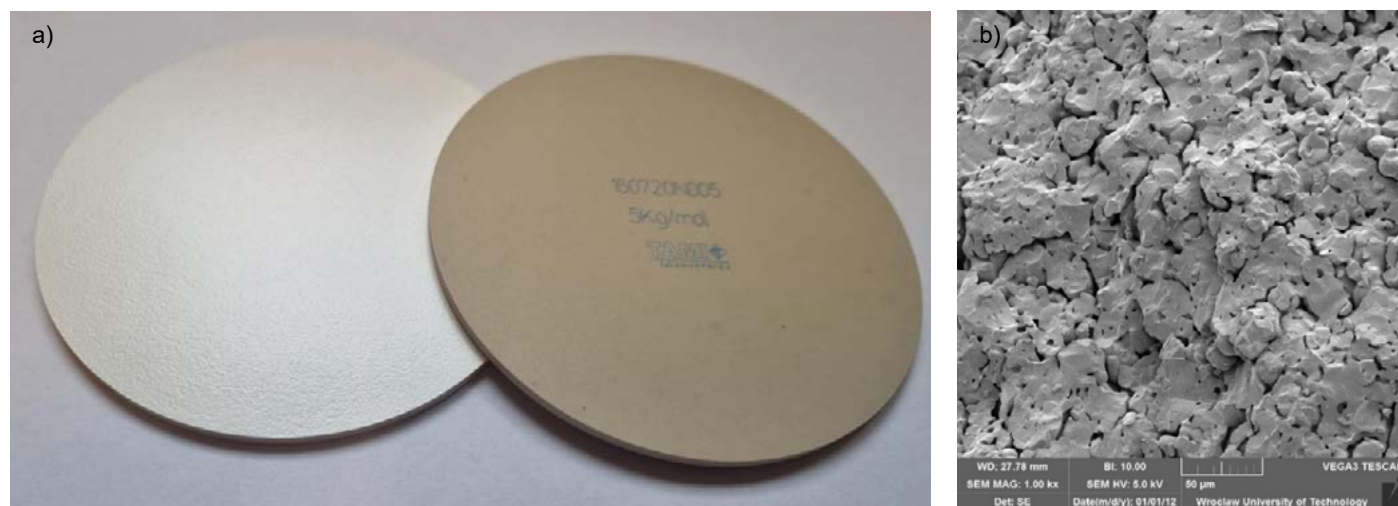
Fig 1. Example photograph of the 5 kDa cut-off flat ceramic membrane used in this study (a) and its SEM image (1000x magnification) (b)
