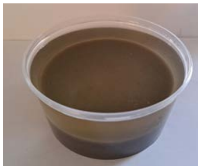
Fig 4. Lack of compatibility of glass with the polyurethane system
