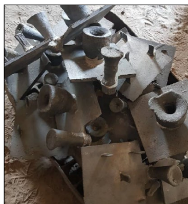
Fig. 1. Hadfield cast samples with the gating and feeding system
