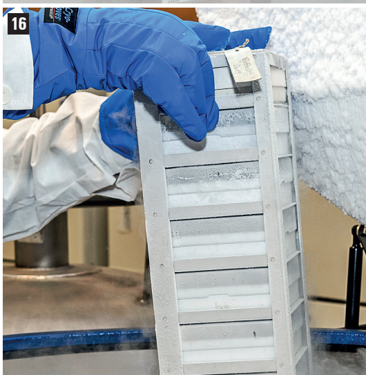
Fot. 16 Cryogenic storage of seeds in the seed bank. Seed samples, placed in cryogenic containers and deposited in cassettes stored in liquid nitrogen ( -196^{\circ}\text{C} ), are conserved using a long-term method that maintains high viability and genetic integrity for decades, minimizing the rate of aging processes
