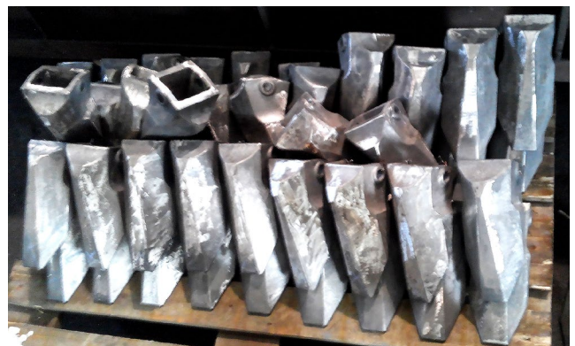
Fig. 13. Good quality tooth castings made using improved technology
