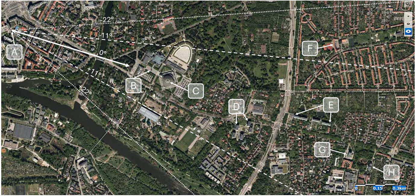
Fig. 2. The situational plan of the experimental setting at Wrocław University of Science and Technology campus at Grunwaldzki Square, where the ENAVI radar was installed (at the balcony of the D-20 building marked as location A), and districts: Dąbie, Śródmieście and Biskupin, where the radar antennas were directed to, with indicated all high-rise architectural objects (locations B–H). Side-lobes of radar antenna are directed to \pm 11^\circ and \pm 22^\circ . Map source: geoportal.gov.pl. Scale 1:10000.
