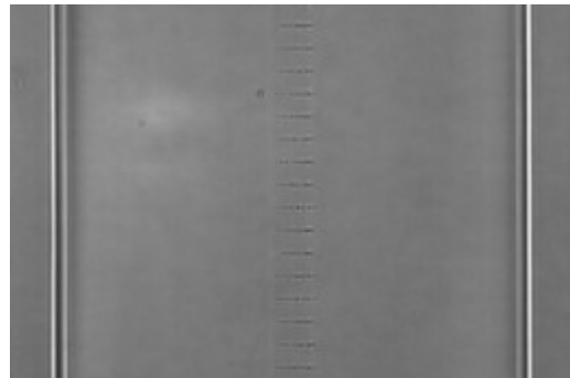
Fig. 1. Microscope image of the fabricated HO-FBG.
