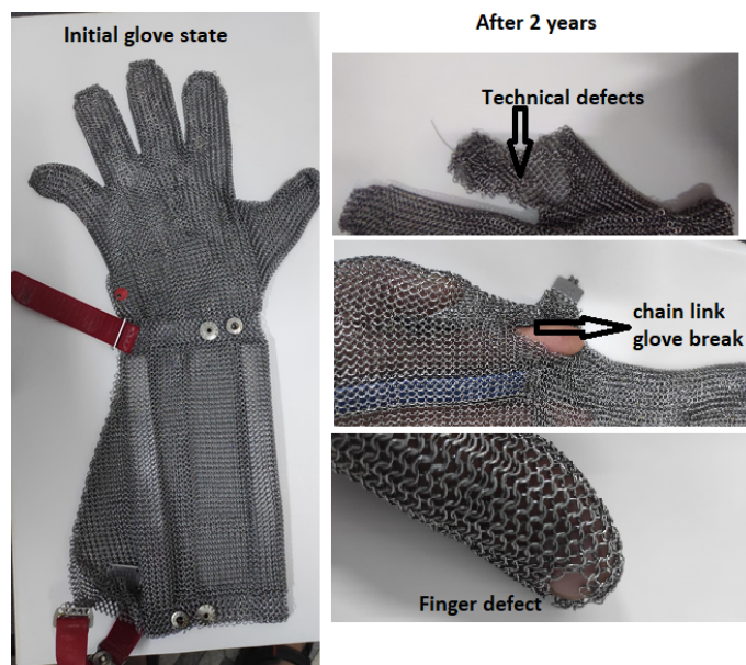
Fig. 1. Metallic protection glove for butchery as initial state and after 2 years of usage
