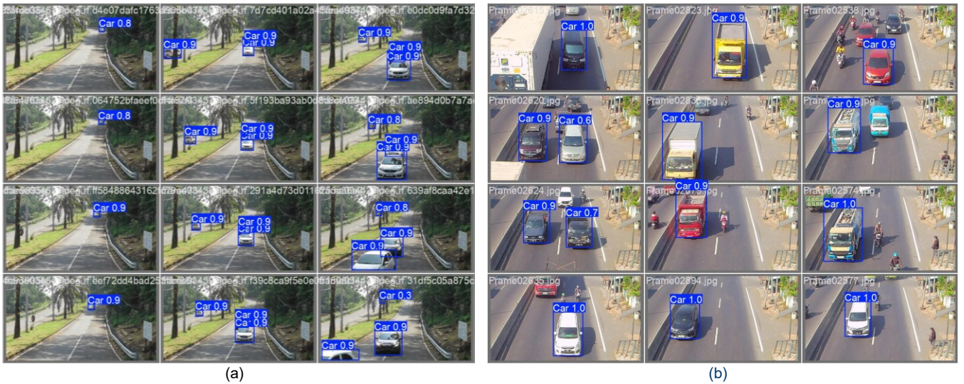
Fig.10. Example of car detection: (a). SLT dataset, (b). SHT dataset
