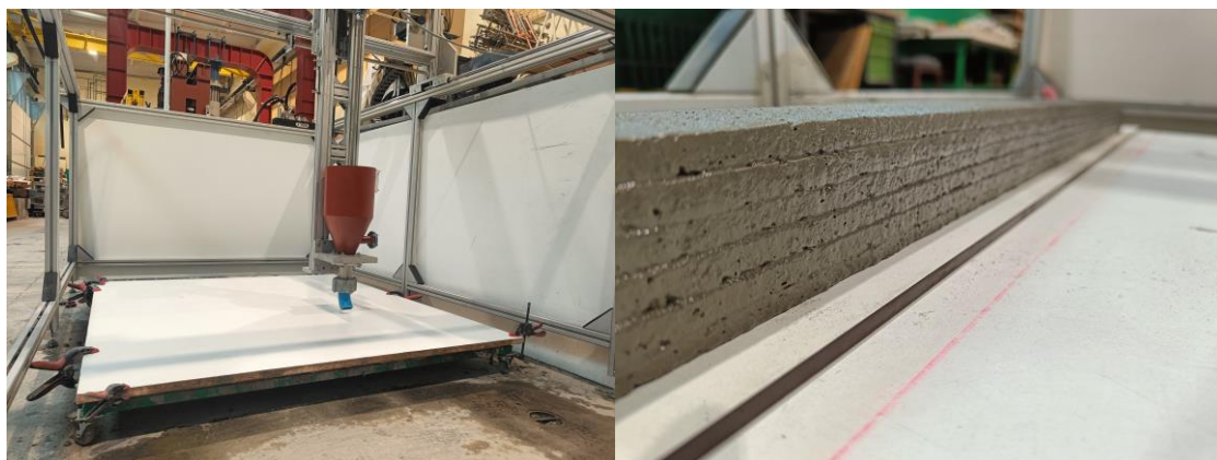
Fig. 1. Samples preparation: 3D printer (left); sample during printing process (right).
