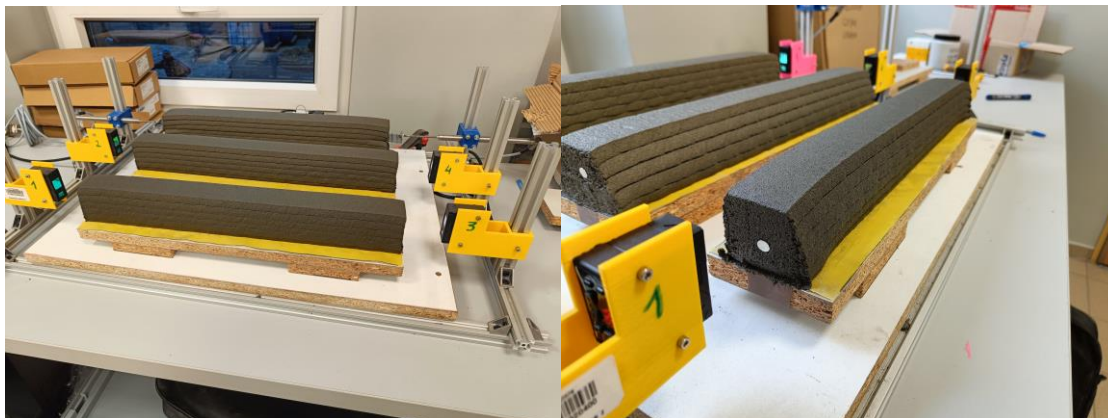
Fig. 3. Measuring shrinkage of 3D printed samples: measuring setup (left); sample with a reference point for laser measurement (right).
