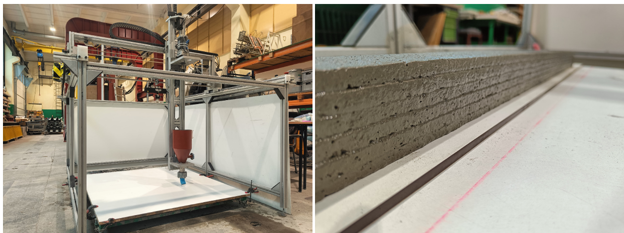
Fig. 1. Samples preparation: 3D printer (left); sample during printing process (right)
