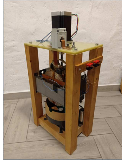
Fig. 17. Photo of the laboratory stand with the investigated transformer
