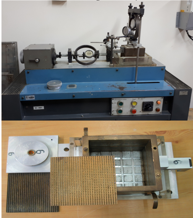
Fig. 2. General view of the AB2A direct shear apparatus and shear box (photo: R. Wojtaszek)
