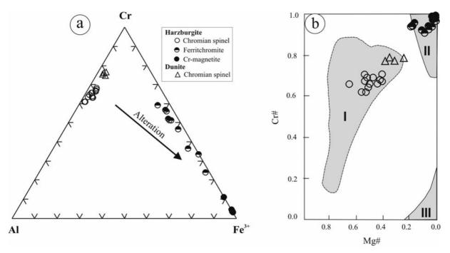
Text-fig. 5. a – Cr–Al–Fe<sup>3+</sup> plot of chromian spinels and their alteration products, and b – Mg# vs. Cr# variation diagram (fields after Roeder 1994 and Mondal *et al.* 2001). Field I: Cr-spinels in mantle peridotites, field II: magnetite from metamorphic rocks, field III: magnetite from unmetamorphosed igneous rocks
