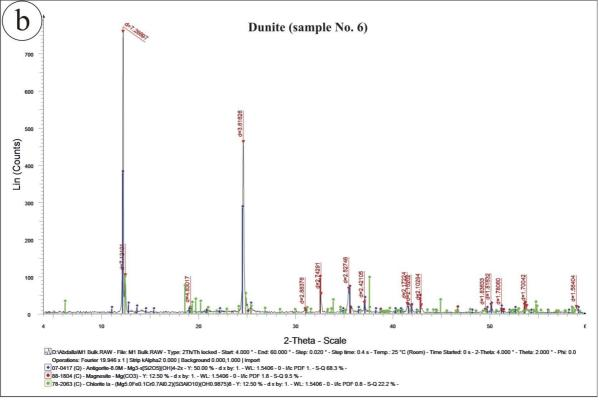
$Text-fig. \ 3. \ a-Chart \ of \ X-ray \ diffraction \ analysis \ in \ the \ serpentinized \ harzburgite, \ and \ b-Chart \ of \ X-ray \ diffraction \ analysis \ in \ the \ serpentinized \ dunite \ du$
