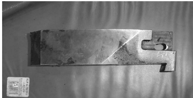
Fig. 2. Standard tool used on wheel-turning lathe
