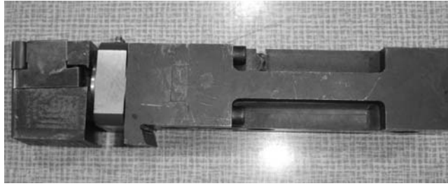
Fig. 3. Special tool with inserted force meter
