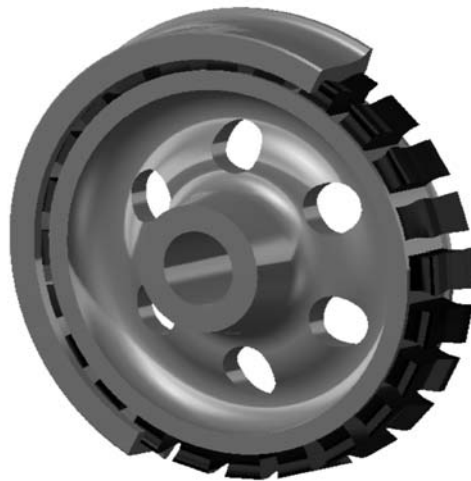
Fig. 1. Pictorial drawing of chosen resilient wheel construction
