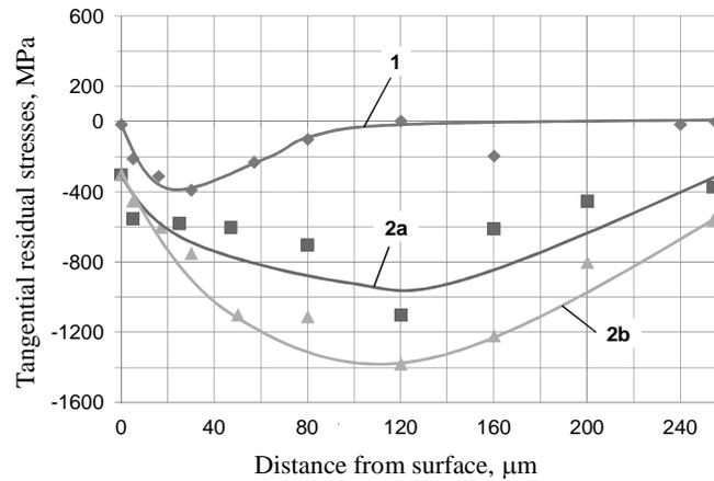
Fig. 7. Distribution of tangential residual stresses for a hard turned and burnished 41Cr4 steel after [4]: 1 – hard turning, 2a – ball burnishing at  $p = 20$  MPa, 2b – ball burnishing at  $p = 40$  MPa
