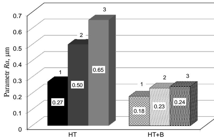
Fig. 2. Comparison of Ra values for hard turned and burnished surfaces.
