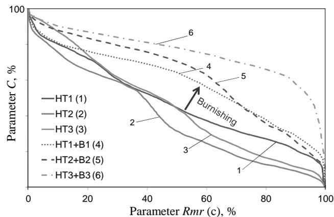
Fig. 4. Material ratio curves for dry hard turning and burnishing operations with variable feeds
