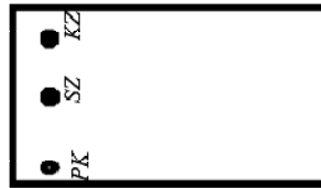
Fig. 5. Position of the measuring points of roughness at the site of primary contact PK, center workpiece SZ and end workpiece KZ
