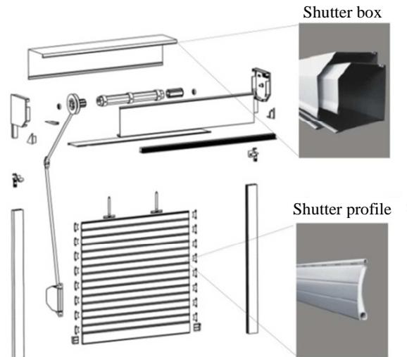
Fig. 1. Roller shutter's components
