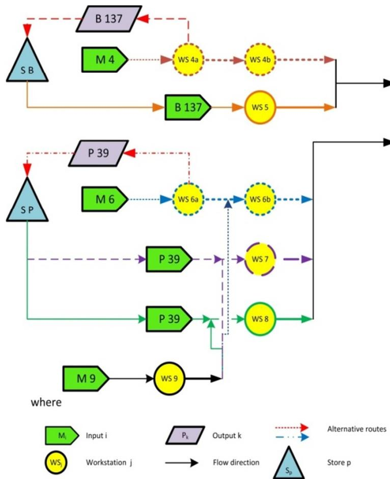
Fig. 2. Alternative routes of the manufacturing process
