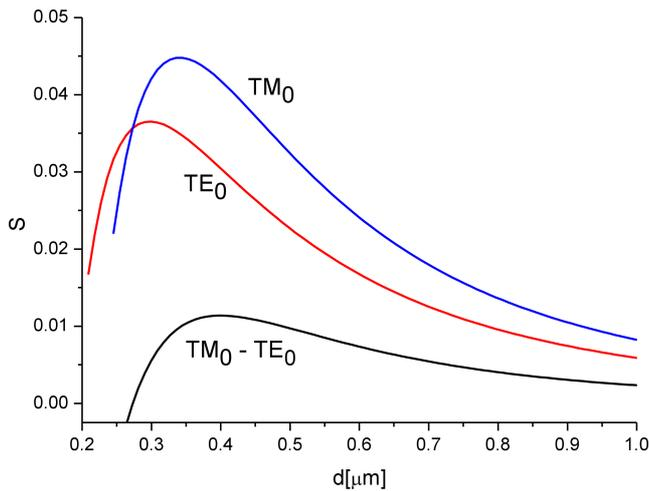
Fig. 2. Sensitivities as a function of the thickness of the waveguide layer concerning a single-mode waveguide
