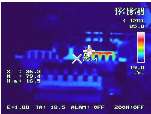
Fig. 14. Temperature distribution of the radiator, hard switching
