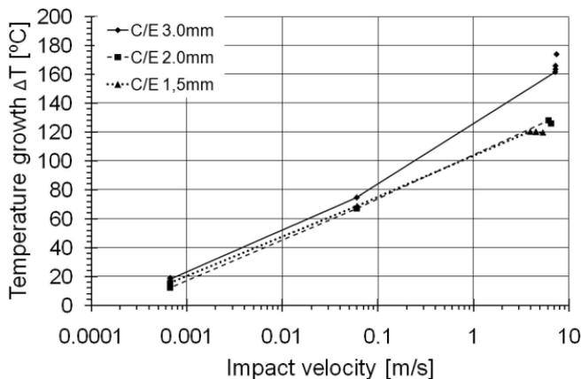
Fig. 6. The influence of load velocity on the temperature growth of the specimens made of C/E composites with different tube wall thickness
