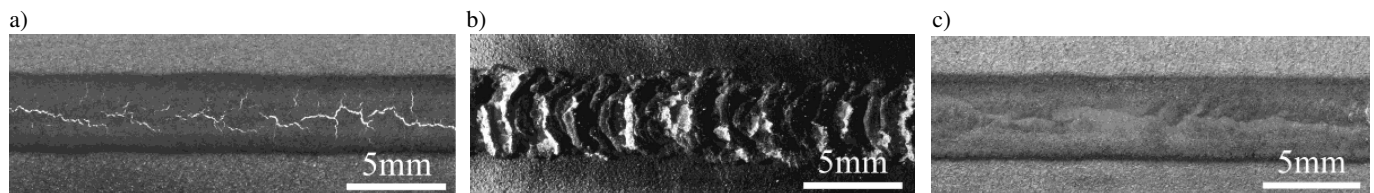
Fig. 6. TIG DC produced weld: (a) without vibrations within the (b) assisted with ultrasonic vibrations in the 0.127 m ( 1/2\lambda ) region, and (c) with vibrations in the 0.1905m region ( 3/4\lambda )
