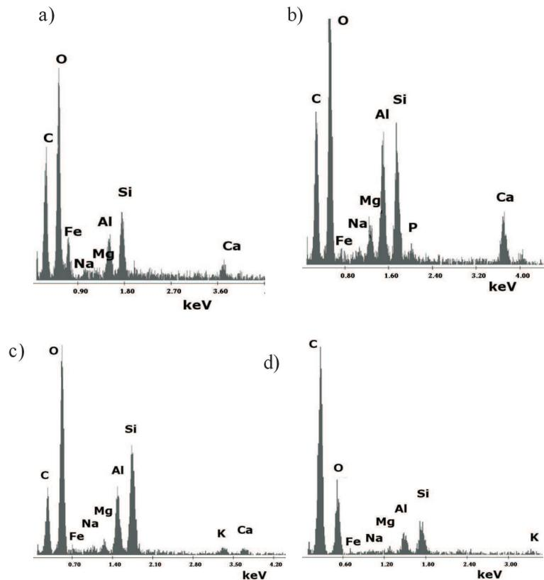
Fig. 3. EDS analysis results in points marked in Fig. 2: a) point 1; b) point 2; c) point 3; d) point 4.
