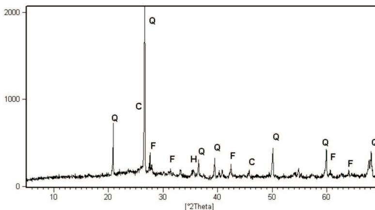
Fig. 1. X-ray pattern of fly ash used (Q –  $\beta$ -quartz, H – hematite, C – carbon, F – iron sulphate).
