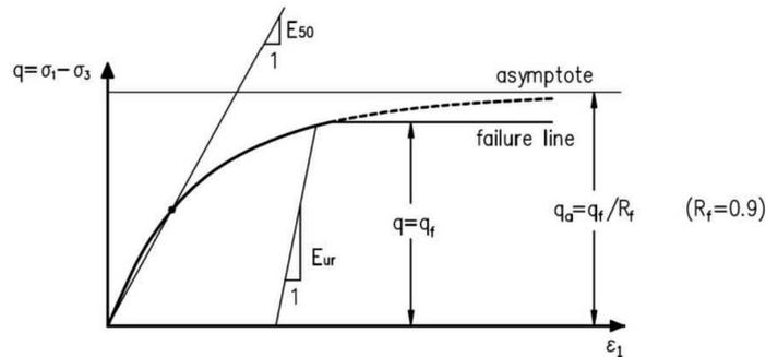
Fig. 3. Hyperbolic stress-strain relationship used in HS model (PLAXIS program).
