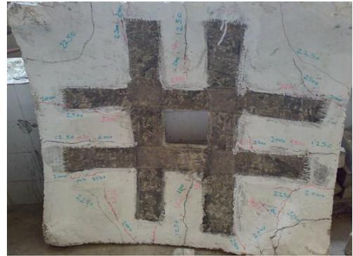
Fig. 20. Crack pattern of shell Strengthened by using 2 layers GFRP (Type 1). [Failure load = 3500 kg]
