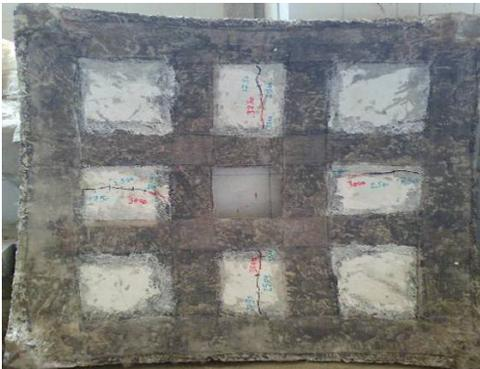
Fig. 21. Crack pattern of shell Strengthened by using 2 layers GFRP (Type 2). [Failure load = 3500 kg]
