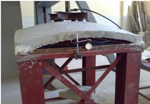
Fig. 7. Shell strengthened by using external tie.
