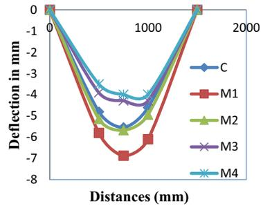
Fig. 16. Deflection Profile of Reference and Strengthened Beams at the Load Levels of 40kN
