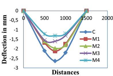
Fig. 15. Deflection Profile of Reference and Strengthened Beams at the Load Level of 20kN
