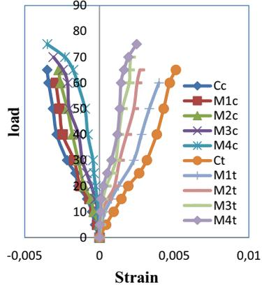
Fig. 8. Load-Compressive and Tensile Strain of Reference and Strengthened Beams
