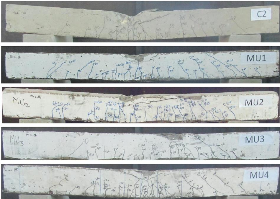
Fig. 18. Failure Crack Pattern of Reference and Strengthened Beams
