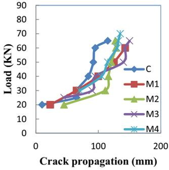
Fig. 11. Load-Crack Propagation of Reference and Strengthened Beams
