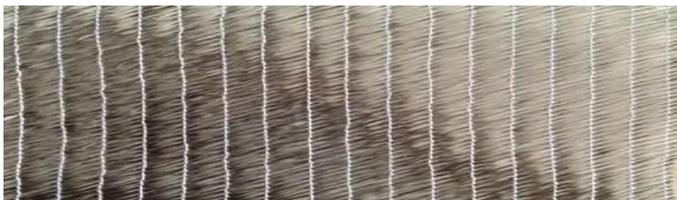
Fig.1. Multi- directional basalt fibre fabric
