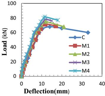
Fig. 5. Load-Central Deflection of Reference and Strengthened Beams
