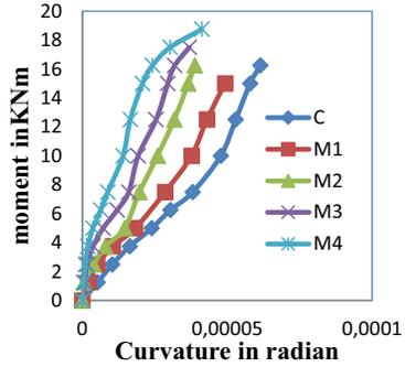
Fig. 7. Moment-Curvature (Strain) of Reference and Strengthened Beams
