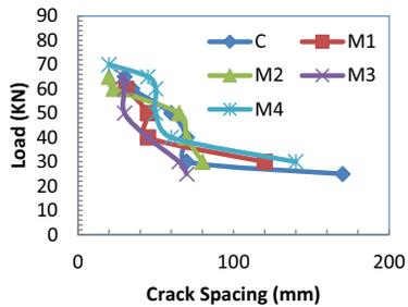
Fig. 10. Load-Crack Spacing of Reference and Strengthened Beams
