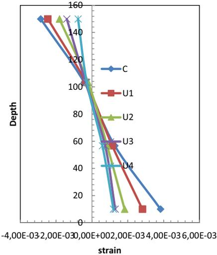
Fig. 12. Compressive and Tensile Strain Profile of Reference and Strengthened Beams at the Load Level of 20kN
