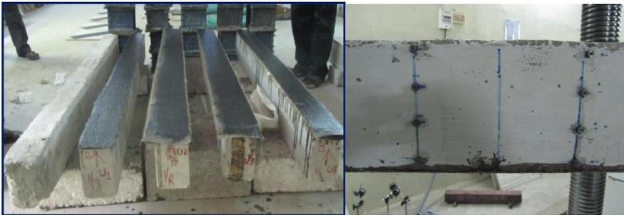
Fig. 3. Wrapped Specimens and Pellets fixation
