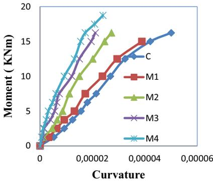
Fig. 6. Moment-Curvature (deflection) of Reference and Strengthened Beams
