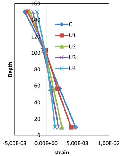
Fig. 13. Compressive and Tensile Strain Profile of Reference and Strengthened Beams at the Load Level of 40kN
