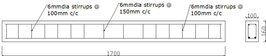
Fig.2. Reinforcement Details of Beams
