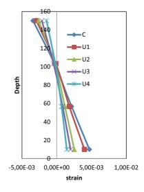
Fig. 13. Compressive and Tensile Strain Profile of Reference and Strengthened Beams at the Load Level of 40kN
