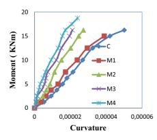
Fig. 6. Moment-Curvature (deflection) of Reference and Strengthened Beams
