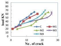
Fig. 9. Load-Number of Cracks of Reference and Strengthened Beams
