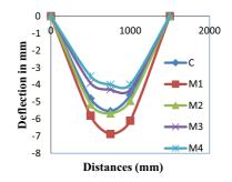
Fig. 15. Deflection Profile of Reference and Strengthened Beams at the Load Level of 20kN
