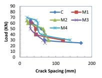
Fig. 10. Load-Crack Spacing of Reference and Strengthened Beams
