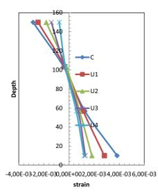
Fig. 12. Compressive and Tensile Strain Profile of Reference and Strengthened Beams at the Load Level of 20kN
