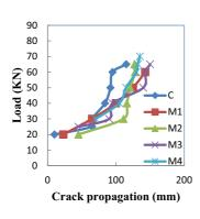
Fig. 11. Load-Crack Propagation of Reference and Strengthened Beams
