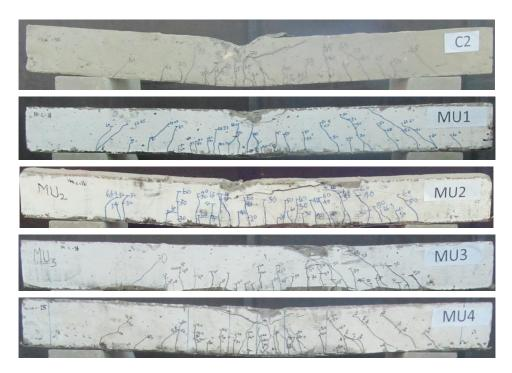
Fig. 18. Failure Crack Pattern of Reference and Strengthened Beams
