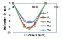
Fig. 17. Deflection Profile of Reference and Strengthened Beams at the Load Level of 60kN
