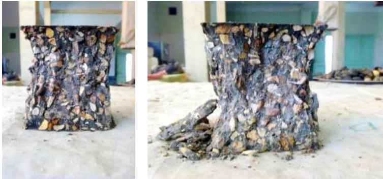
Fig. 1. SC samples after compressive strength test and immersion time for 6 months.
