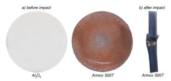
Fig. 8. Panel components before and after impact
