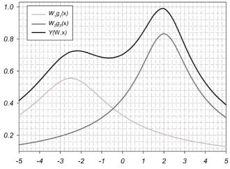
Fig. 4. Approximation with radial neural network
