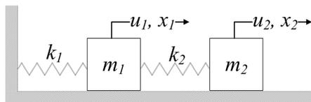
Figure 8. Schematic image of double spring-mass system.
