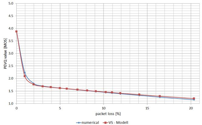
Fig. 9. QoS values as functions of packet losses gained from different measuring methods for the Codec H.264/AVC and the MPEG-2-TS, a burst size of “1” and an encoding rate of 2125 kbps
