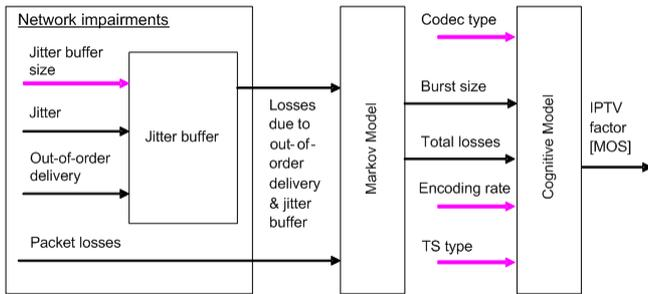
Fig. 1. Block diagram for the IPTV model
