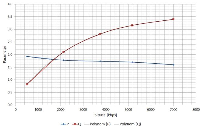
Fig. 5. Approximation of parameters P and Q as functions of the encoding rate for the codec H.264/AVC and the MPEG-2-TS
