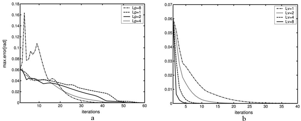
Figure 7. a) The profiles of maximal tracking error for  $K_v = 8$ ,  $L_v = 0$  and  $K_p = 1$ ,  $L_p = 1, 2, 4, 8$ ; b) The profiles of maximal tracking error for  $K_v = 8$ ,  $L_v = 1, 2, 4, 8$  and  $K_p = 1$ ,  $L_p = 2$ .
