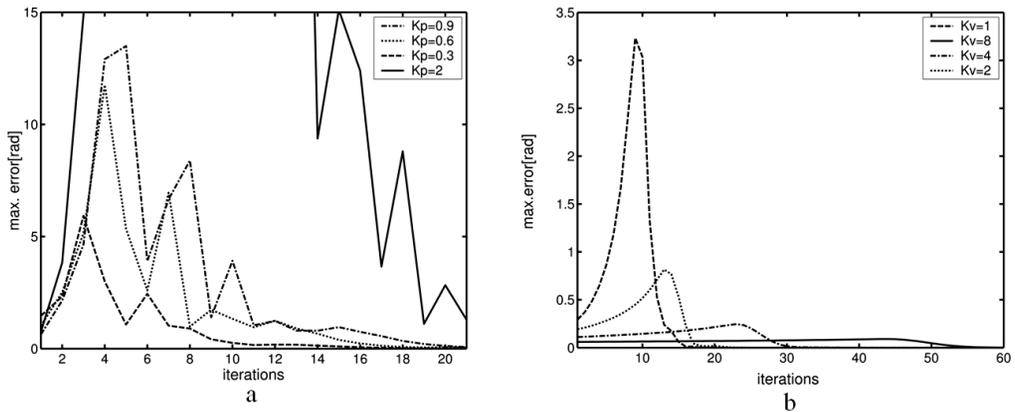
Figure 6. a) The profiles of maximal tracking error  $e_l^{\max}$  for  $K_v = 0$ ,  $L_v = 0$ ; and  $K_p = 0.3, 0.6, 0.9, 2$ ,  $L_p = 0$  b) The profiles of maximal tracking error for  $K_v = 1, 2, 4, 8$ ,  $L_v = 0$  and  $K_p = 0$ ,  $L_p = 0$ .
