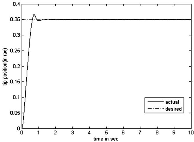
Figure 12. Tip position response for BFO optimized FLC.
