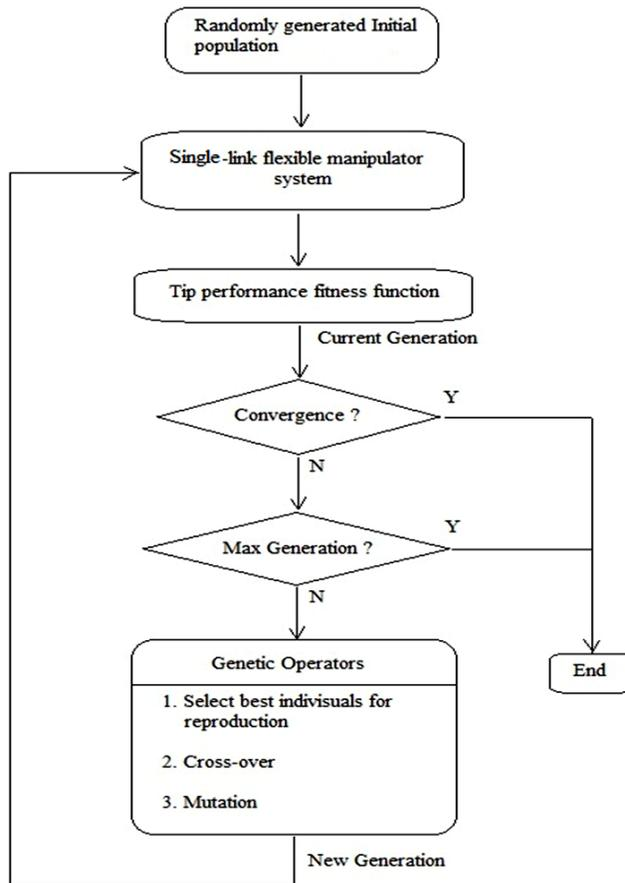
Figure 6. Genetic algorithm optimization process.
