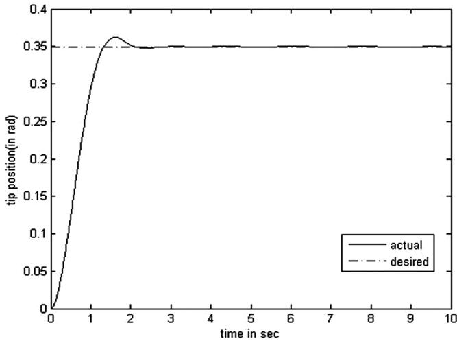
Figure 11. Tip position response for GA optimized FLC.
