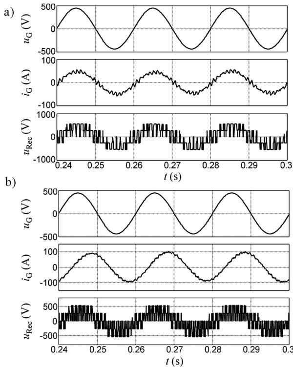
Figure 5. Generator output phase voltage  $u_G$  and current  $i_G$ , and input phase voltage  $u_{Rec}$  of the PWM rectifier: a)  $\varphi = 0^\circ$ ,  $\psi = 9.7^\circ$ , b)  $\varphi = 60^\circ$ ,  $\psi = 12.5^\circ$ .
