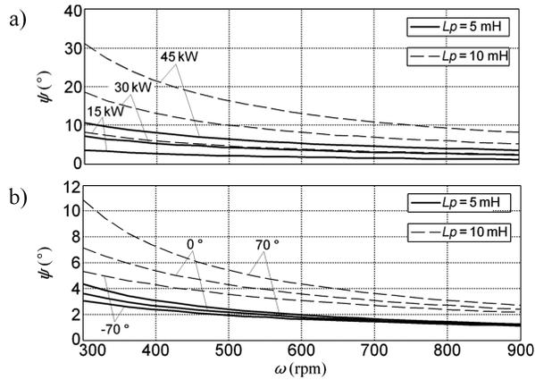
Figure 3. The angle  $\psi$  as a function of the rotational speed  $\omega$  of the turbine – PM generator unit for assumed: a) power  $P$  ( $\varphi = 0^\circ$ ), b) phase angle  $\varphi$  ( $P = 30\text{kW}$ ).
