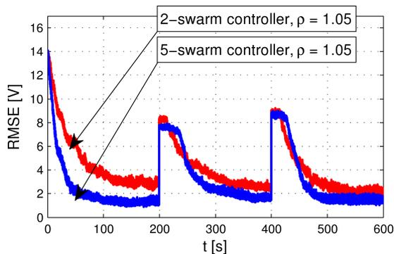
Fig. 7. Comparison of the RMSE graphs for the 2-swarm and 5-swarm controllers
