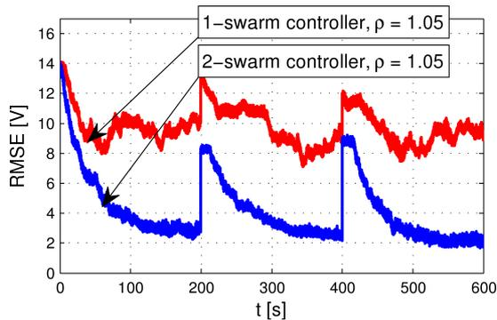
Fig. 6. Comparison of the RMSE graphs for the single-swarm and 2-swarm controllers
