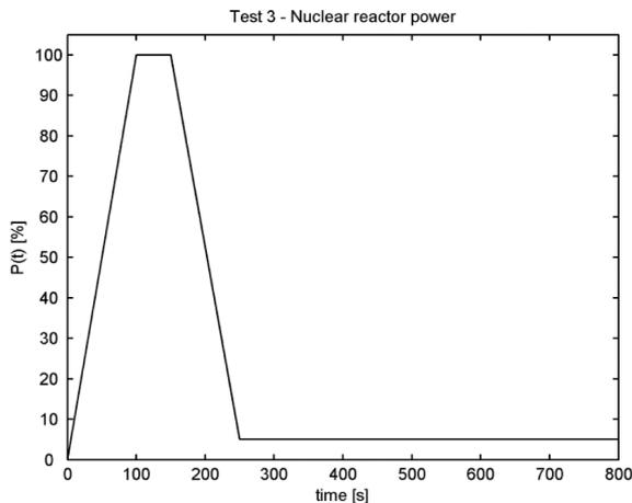
Fig. 12. Thermal power change – positive and negative slope of power curve.
