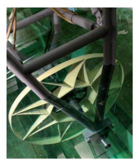
Fig. 3. CMMCT with support structure in a water towing tank
