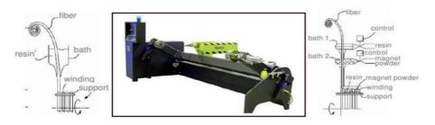
Fig. 5. Fiber wetting with one bath (left), example of multiple axis winding machine (center), controlled alternative fiber wetting with two baths (right)
