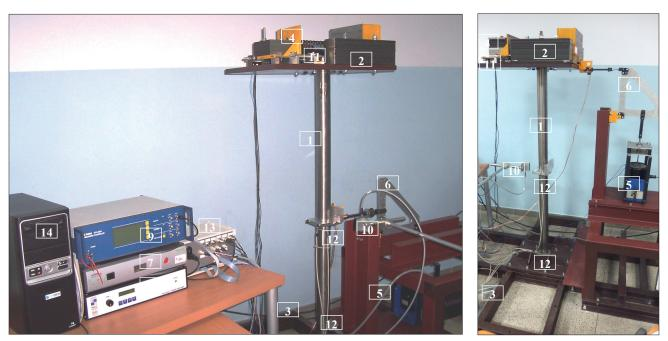
Fig. 2. Laboratory test rig: excitation applied to the tower midpoint (left) or to the nacelle (right)
