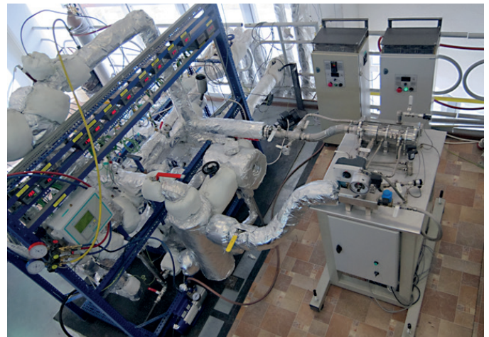
Fig. 3. Test rig for testing heat exchangers and expanders (including vapour micro-turbines) [12]
