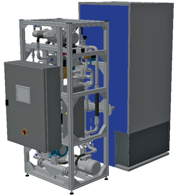
Fig. 5. Three-dimensional CAD model of the CHP ORC energy system
