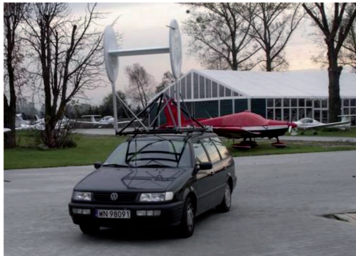
Fig. 25. Dynamic testing of EB-3
