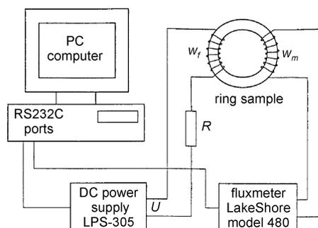
Fig. 2. The block diagram of the computer controlled experimental setup
