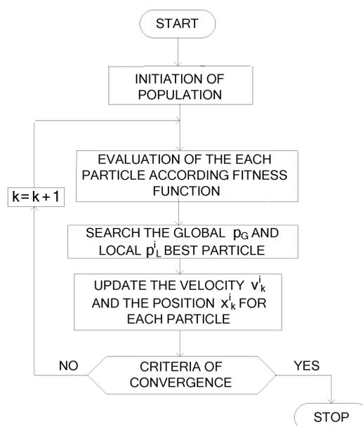
Fig. 1. The block diagram of the PSO algorithm
