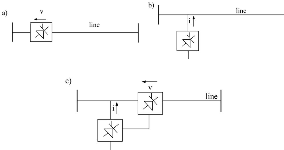
Fig. 2. Basic type of FACTS devices: a) series controllers; b) shunt controllers; c) series and shunt controllers
