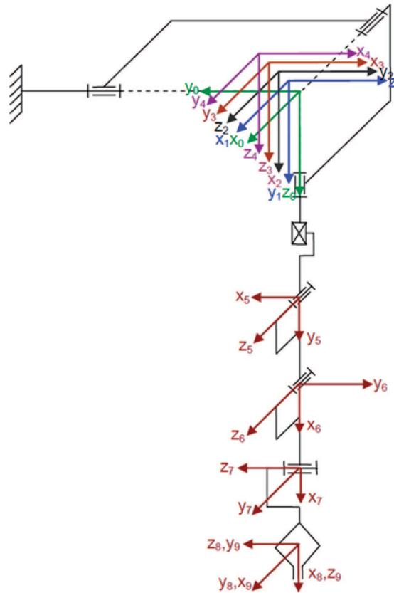
Fig. 7. The model of the RobIn Heart robot
