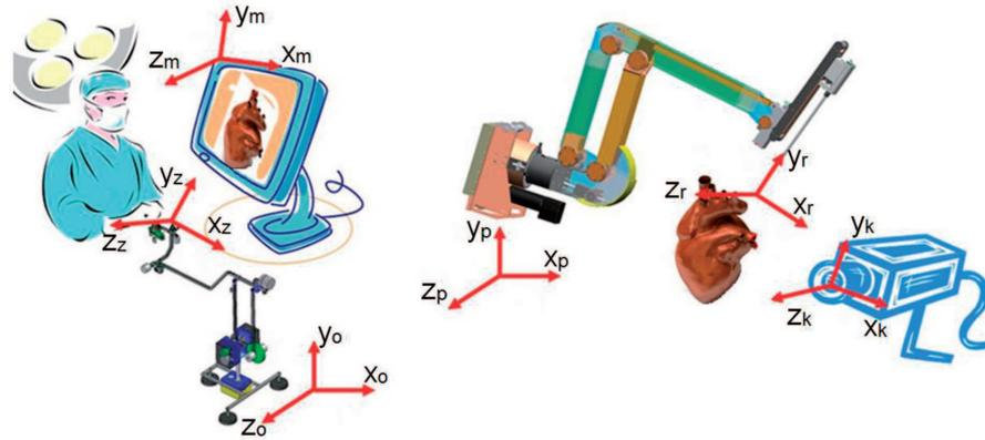
Fig. 6. Coordinates systems associated with each component of RobIn Heart telemanipulator where:  $x_o, y_o, z_o$  – base coordinate system of master manipulator,  $x_m, y_m, z_m$  – coordinate system of monitor,  $x_z, y_z, z_z$  – coordinate system of master's handle,  $x_p, y_p, z_p$  – base coordinate system of robot,  $x_r, y_r, z_r$  – coordinate system of robot's tool (TCP),  $x_k, y_k, z_k$  – coordinate system of camera
