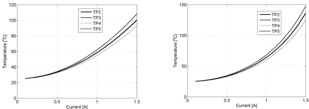
Fig. 7. Static temperature of the chosen actuator points vs. current density value:
