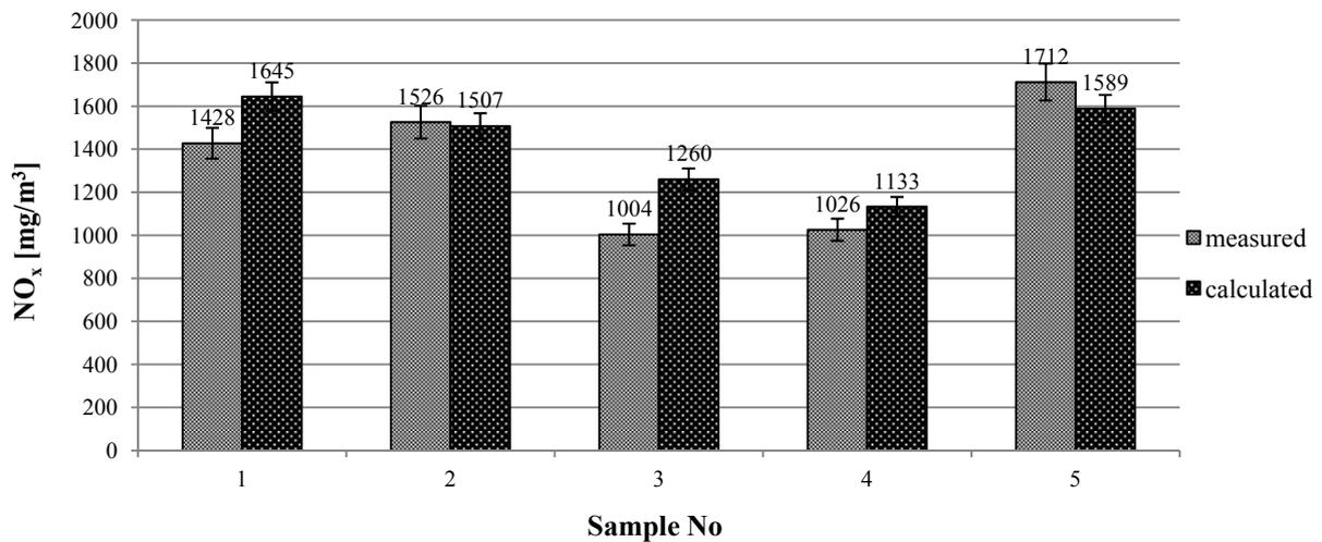
Fig. 12. Average concentrations of NO<sub>x</sub>, the investigation and the resulting calculations comparison;
