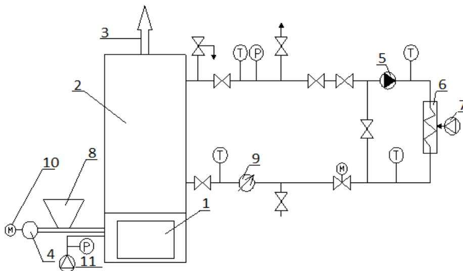
Fig. 1. The main diagram of biomass combustion;
