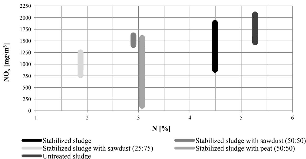
Fig. 9. NO<sub>x</sub> dependence from total nitrogen (N) quantity
