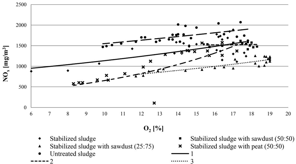
Fig. 8. Variations of NO<sub>x</sub> concentrations in samples;
