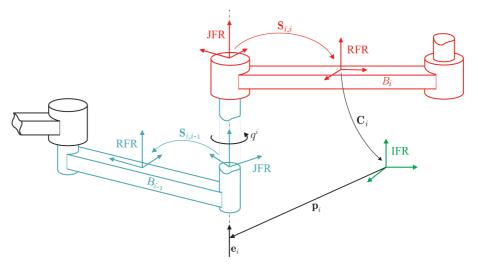
Fig. 4. Relative kinematics of adjacent bodies
