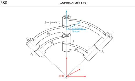
Fig. 6. Cut-joint and reference frame for spherical 4-bar mechanism. Shown is the reference configuration
