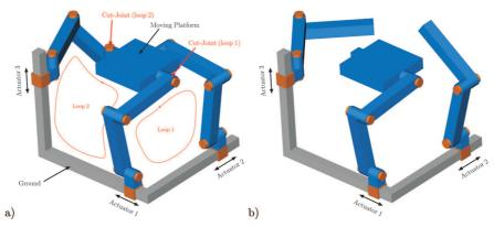
Fig. 7. a) Independent fundamental loops for the 3PRRR PKM. b) Tree-topology MBS model with 10 generalized coordinates
