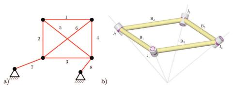
Fig. 1. a) A topologically overconstrained planar mechanism, b) A geometrically overconstrained spherical mechanism
