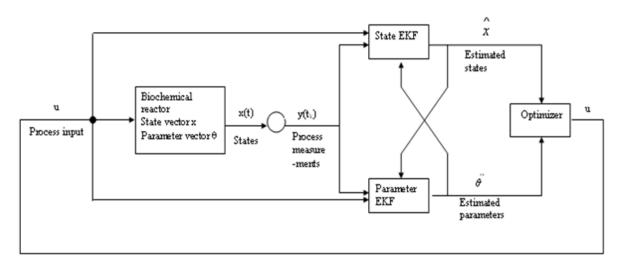
Fig. 1. Two level EKF assisted on-line optimisation control scheme
