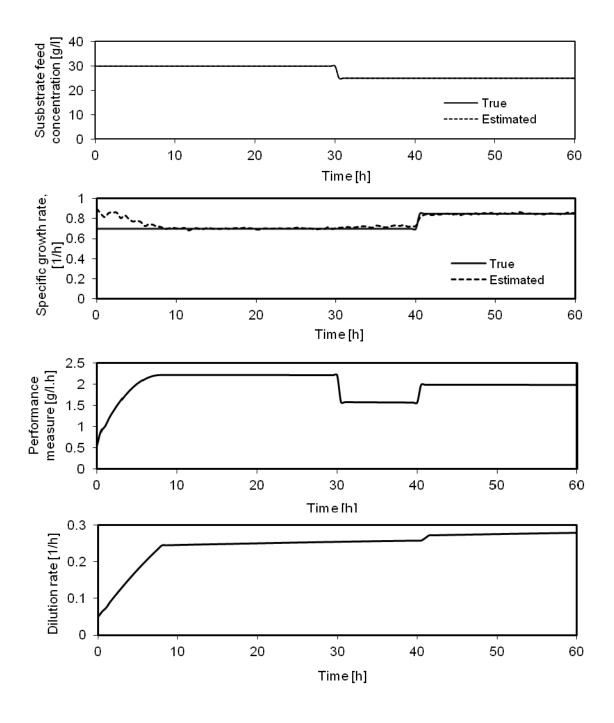
Fig. 5. Results of two-level EKF assisted online optimiser in the presence of parameter uncertainties
