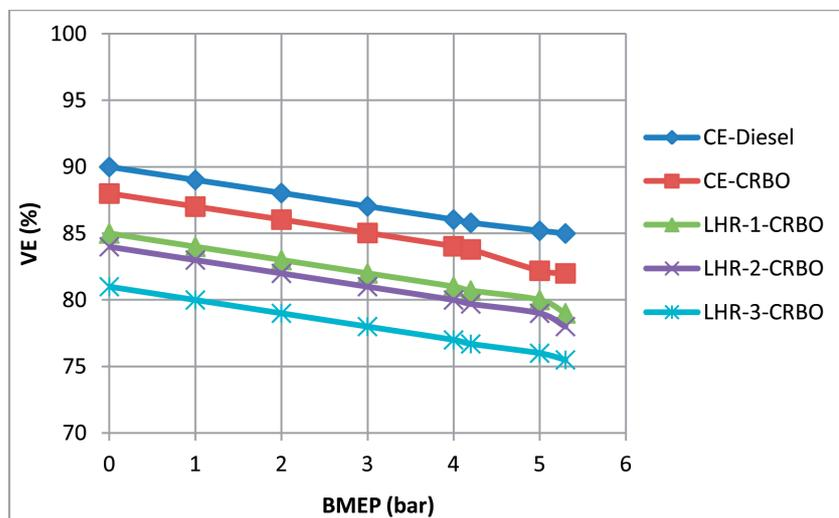
Fig. 6. Variation of volumetric efficiency (VE) with BMEP in different versions of the engine with CRBO operation at an injector opening pressure of 190 bar
