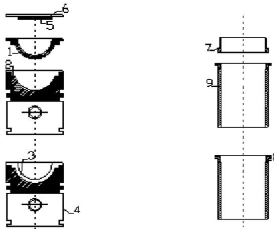
*Insulated piston      Insulated liner      Ceramic coated cylinder head*
