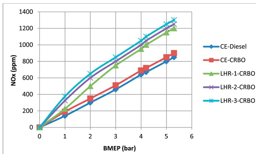
Fig. 8. Variation of NO<sub>x</sub> levels with BMEP with test fuels in different versions of the engine with CRBO operation at an injector opening pressure of 190 bar
